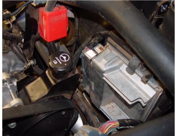
7. Coat the connector terminal with dielectric grease and insert it into position 71 on the C1 Connector. You will need to insert a sharp object to pierce the rubber seal on the connector. Push the terminal far enough down and you will feel the lock engage. Pull back slightly to ensure that it is locked in place.
