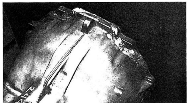
(71-23) Welded but distorted G56 case at bell housing area.
